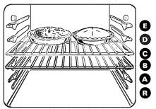
place most foods in the middle of the oven, on either shelf position B or C. See the chart for suggested shelf positions. If you think an adjustment is necessary, see the Adjust the Oven Thermostat section. It gives easy *Do It Yourself* instructions on how to adjust the thermostat.
