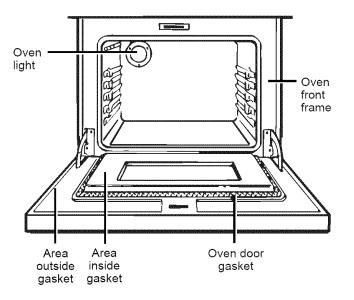
**3.** Clean spatters or spills on the oven front frame, and the oven door outside the gasket with a dampened cloth. The oven front frame and the oven door outside the gasket do not get cleaned by the self-clean cycle. On these areas use detergent and hot water or a soap-filled steel wool pad. Rinse well with a vinegar and water solution. This will help prevent a brown residue from forming when the oven is heated. Buff these areas with a dry cloth. Do not clean the gasket.
