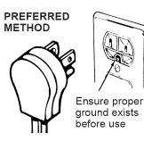
wall receptacle to minimize the possibility of electric shock hazard from this appliance. The customer should have the wall receptacle and circuit checked by a
