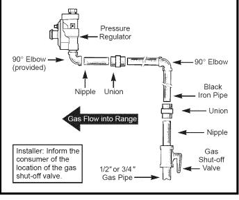
Flexible Connector and Rigid Pipe Hookups for Models Equipped with Standard Twin Burners
