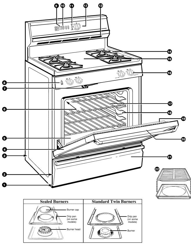
Your range is equipped with one of the two types of surface burners shown above.
