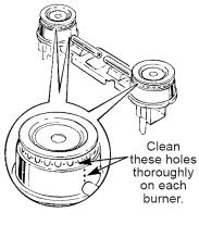
You should clean the surface burners routinely, especially after bad spillovers, which could clog these holes. Wipe off surface burners. If heavy spillover occurs, remove the surface burners from the range. Burners lift out for cleaning. Lift up the cooktop and then lift out the surface burners.
