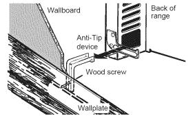
**5.** Slide the range against the wall, and check for proper installation by grasping the front edge of the cooktop and carefully attempting to tilt the range forward.
