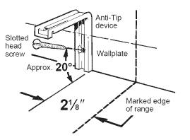
**2.** Locate the outside edge of the device  $2\frac{1}{2}$  toward the center of the range from the marked edge of the range.
