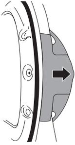
2. Gently pull the plastic cover out and down. This unsnaps the plastic hinge cover from the inside door assembly.
