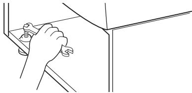
**10.** When the washer/dryer is level, use a 9/16" (14.3 mm) open-end wrench to securely tighten all four locknuts against the pedestal. The locknuts must be tightened.
