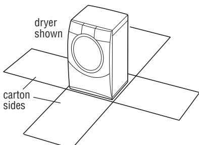
**2.** Lay washer/dryer on its back.
