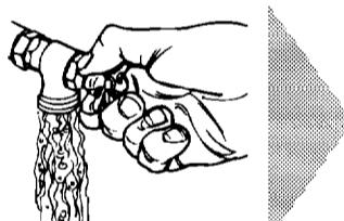
Run water through both faucets into a bucket to get rid of particles in the water lines that might clog hoses. Mark the hot water faucet.
