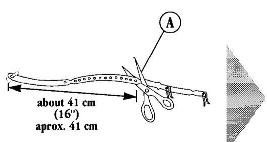
After shipping strap has been removed from washer, look for the words "cut here" marked on the shipping strap, about 41 cm (16 inches) from the plug end. Cut the shipping strap at this mark (A).
