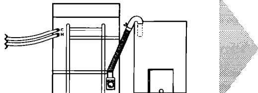
If a longer drain hose is needed, drain hose extension kit (Part No. 285702) is available from authorized parts distributors. If drain hose must be shortened, use hose kit (Part No. 285442).
