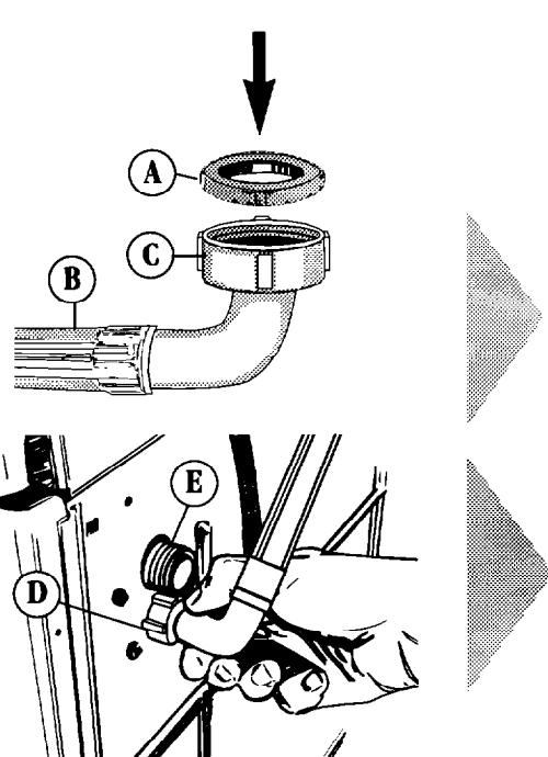
Insert a flat washer (A) into each end of the inlet hoses (B). Check that washers are firmly seated in couplings (C).
