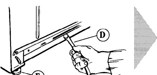
Pull firmly to remove the other end of the shipping strap (D) from the back of the washer to release self-leveling legs (E).
