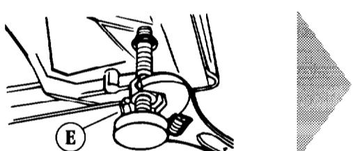
If washer is not level, adjust the front legs (E) up or down. Repeat above step.
