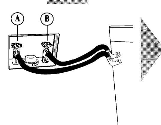
Attach bottom hose from the inlet marked "H" to hot water faucet (A). Attach top hose from the inlet marked "C" to cold water faucet (B). Adapters maybe necessary to connect hoses to faucets.
