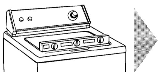
Tilt washer forward, raising back legs 2.5 cm (1 inch) off of floor to adjust rear self-leveling legs. Drop washer to floor. Check levelness of the washer by placing a carpenter's level on top of the washer, first side to side; then front to back.
