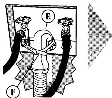
If the water inlet faucets and drain standpipe are recessed, put "hook" end of drain hose (E) in standpipe. Tightly wrap the shipping strap (F) around the drain hose and faucet body (not the handle or stem). Push plug into the nearest hole in the shipping strap.
