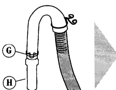
If drain hose does not fit into standpipe or is being placed over the edge of a laundry tub, open other drain hose clamp with pliers and place clamp over rubber end of drain hose (G).
