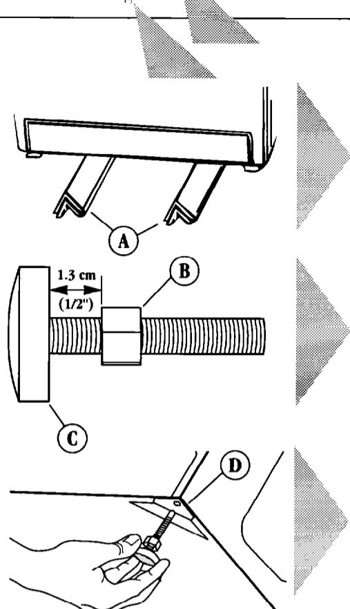
Stack two corner posts (A) on top of each other. Tilt washer backwards and slide corner posts under washer 7.6 cm (3 inches) from each side of washer as shown.
