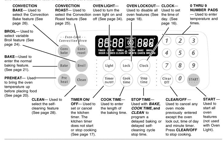
Minimum and Maximum Control Pad Settings All of the features listed have minimum and maximum time or temperature settings that may be entered into the control. An ENTRY acceptance beep will sound each time a control pad is touched (the Oven Lockout pad is delayed by 3 seconds).
