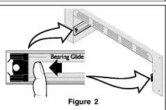
Removing and Replacing the Warming Drawer (Stainless Steel models only)
