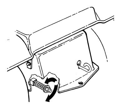
ROTATE ADJUSTING NUT CLOCKWISE TO INCREASE BRAKING OR COUNTER CLOCKWISE TO DECREASE BRAKING
