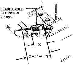
**8.** (33" Deck) To adjust tension, remove extension rod mounting bolt and nut. See Figure 4.4.
