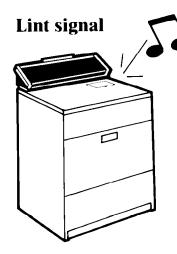
Clean lint screen **before each load.** If you neglect to clean your lint screen, the signal will sound. The (whistle tone) signal lets you know the air flow is being restricted. Restricted air flow reduces drying efficiency.
