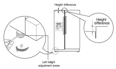
If the freezer compartment door is higher than the refrigerator compartment door Level the door by inserting flat (-type) driver into the groove of the right height adjusting screw and rotate it clockwise (①).
