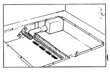
To determine if the bottom (oven) burner flame is proper, remove the oven bottom (see page 18) and the burner baffle. The flame should have 1/2" to 3/4" blue cones with no yellow tipping. When the baffle is back in place, the flame will resettle.
