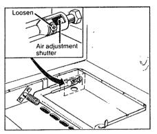
The shutter for the bottom (oven) burner is near the back wall behind the storage drawer. To adjust the flow of air to either burner, loosen the Phillips head screw and rotate the shutter to allow more or less air into the burner tube as needed.
