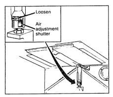
The air adjustment shutter for the top (broil) burner is in the center of the rear wall of the oven.
