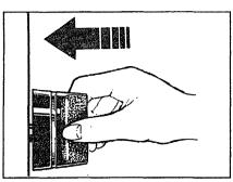
Push the control knob in and turn it to LITE. You will hear a little clicking noise—the sound of the electric spark igniting the burner.
