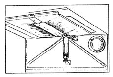
The flame for the top (broil) burner should be steady with approximately 1-inch blue cones and should not extend out over the baffle edges.
