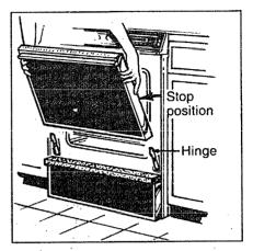
To remove the door, open it a few inches to the special stop position that will hold the door open. Grasp firmly on each side and lift the door straight up and off the hinges.
