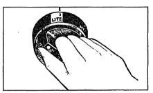
After the burner ignites, turn the knob to adjust the flame size.
