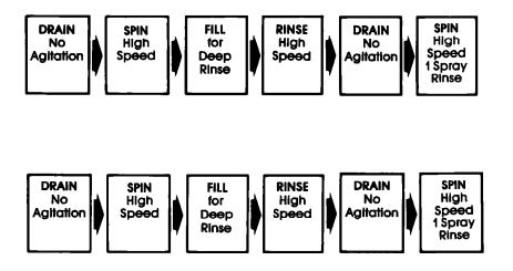
\* IMPORTANT: THE WASHER WILL PAUSE BRIEFLY AT DIFFERENT TIMES IN EVERY CYCLE. These pauses are normal. They allow for the reversing of the motor and normal washer operations.
