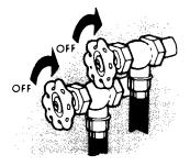
WHEN NOT WASHING, keep both water faucets turned off. This takes the pressure off the water inlet valve and hoses.
