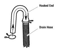
**STEP 3.** Put hooked end of drain hose into laundry tub or standpipe. Check for proper length of drain hose. Rotate hook to eliminate kinks.
