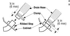
c. Open clamp. Twist hose back and forth while pushing down onto drain connector at the bottom of the washer. Continue until hose contacts the ribbed stop on the cabinet.
