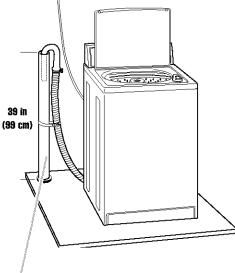
**Standpipe drain system:** Needs a 2 in (5 cm) minimum diameter standpipe with minimum carry-away capacity of 17 gal (64 L) per minute. Top of standpipe must be at least 39 in (99 cm) inches above floor and no higher than 96 in (2.4 m) from bottom of washer.
