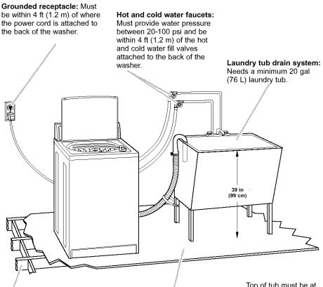
**Support:** Floor must be sturdy enough to support a total weight of 315 lbs (143 kg) (including washer, water, and load weight). Level floor: Maximum allowable slope under entire washer – 1 in (2.5 cm). Top of tub must be at least 39 in (99 cm) above floor and no higher than 96 in (2.4 m) from bottom of washer.
