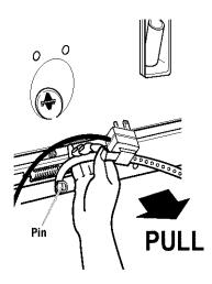
**STEP 3.** Cut the shipping strap about 16 inches (40 cm) from plug end. Look for the words "CUT HERE." Discard end with the cotter pins. **Slide remainder of shipping strap free from the electrical plug.** You will use this to secure the drain hose.
