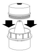
**STEP 7.** Replace the dispenser on the agitator; press firmly to snap into place.
