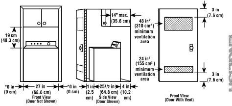
\*Additional clearance for wall, door and floor moldings may be required. To reduce transfer of washer sounds, a clearance of 1 in (2.5 cm) on the sides of the washer is recommended.
