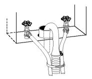
If the water faucets and drain standpipe are recessed, put hooked end of drain hose in standpipe. Tightly wrap the shipping strap around the drain hose and water inlet hoses (not the handles or stems). Push fastener into the nearest hole in the shipping strap.
