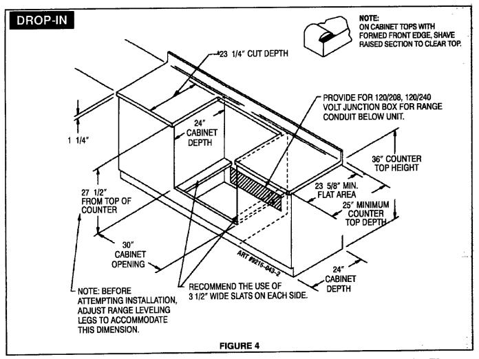
\* When replacing an existing unit, a maximum of 23 1/2" is acceptable. If the cut depth exceeds 23 1/2", use filler kit (K70 Fill).
