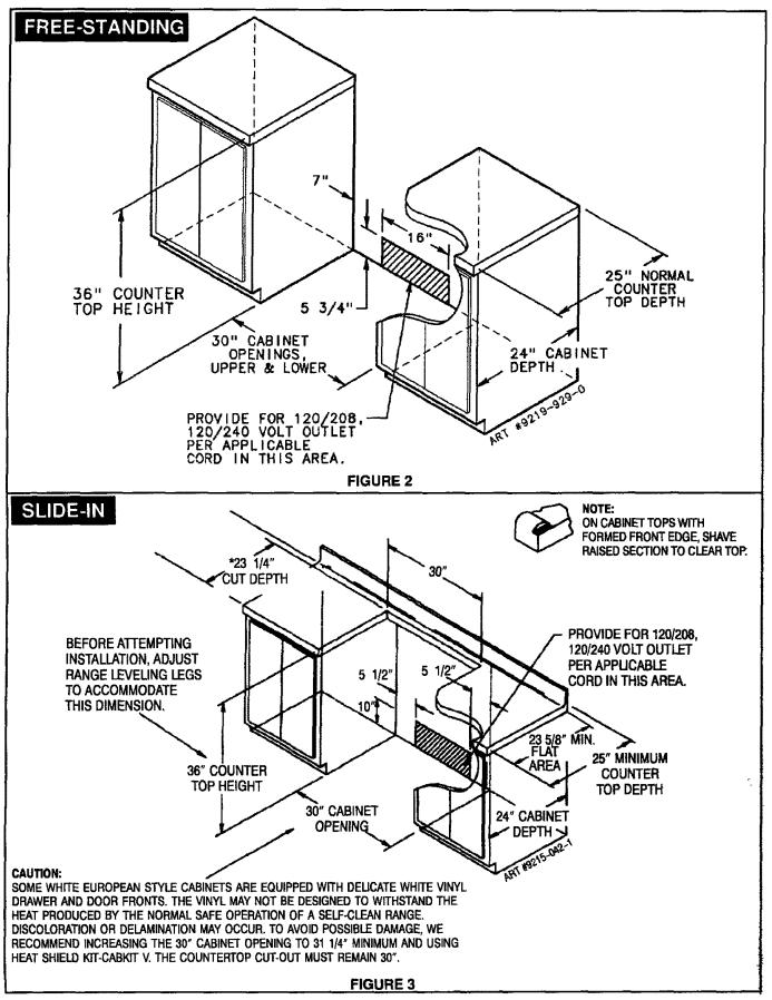
\* When replacing an existing unit, a maximum of 23 1/2" is acceptable. If the cut depth exceeds 23 1/2", use filler kit (K70 Fill).
