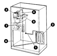
Cubes fall through the chute in the door when the dispenser pad is pressed.
