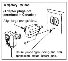
cover screw does not ground the appliance unless the cover screwis metal, and not insulated, and the wall outlet is grounded through the house wiring. You should have the circuit checked by a qualified electrician to make sure the outlet is properly grounded.
