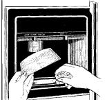
Do not pour water in the spill shell because it is not self drainingpour it in the kitchen sink. The shelf and its grille should be cleaned regularly accord in: to Care and Cleaning Press here to remove grille in structions. The grille is easily removed by pressing on the back right corner.
