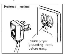
Have the wall outlet and circuit checked by a qualified electrician to make sure the outlet is properly grounded.
