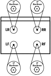
To prevent leakage, make sure the orifice spuds are securely screwed into the gas supply tubes.
