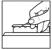
, clean them with a straight pin. Do not enlarge or distort the port. Do not use a wooden toothpick. If the burner needs to be adjusted, call a qualified technician for service. 5. After cleaning the gas tube opening and ports,
