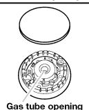
replace the burner cap. To replace the burner cap, make sure the alignment pins on the cap are properly aligned with the burner base.
