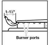
size and shape as shown. A good flame is blue in color. If the flames are not burning at all ports, you may need to clean the burner ports.
