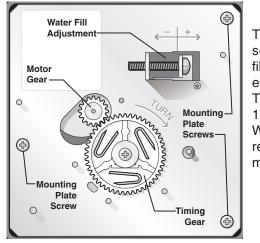
The water fill adjustment screw will change the fill time. One full turn is equal to 20cc (.68 oz.). The correct fill is 102 to 130cc (3.4 to 4.3 oz.). When a water valve is replaced, the fill volume must be checked.
