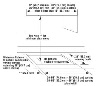
Note: 24" (61 cm) minimum when bottom of wood or metal cabinet is protected by not less than 1/4" (6.4 mm) flame retardant millboard covered with not less than No. 28 MSG sheet steel, 0.015" (0.4 mm) stainless steel, 0.024" (0.6 mm) aluminum or 0.020" (0.5 mm) copper.
