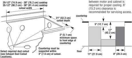
Install rear wall junction box in shaded area. Darker shaded area is preferred.
