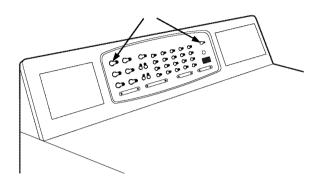
**For dryers:** Using the old overlay as a reference, press and hold the **Air Dry** button in the lower left and the **High** heat button in the upper right of the control panel. After 3 seconds, all lights on the control panel will light up.
