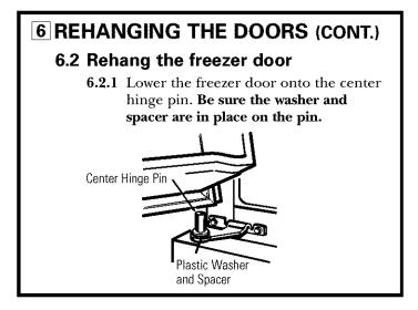
**6.2.2** Tilt the door toward the cabinet, lifting the top hinge so the pin fits into the socket on the top of the door.
