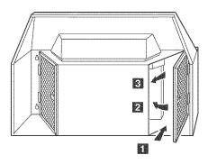
Make sure tabs are toward outside and bottom. Insert aluminum filter into upper track , push in 2 and pull down 3.
