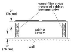
**3.** If cabinet has recessed bottom, add wood filler strips on each side. Locate screws to attach filler strips in locations shown.
