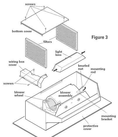
**6** Remove bottom cover screws and bottom cover.
