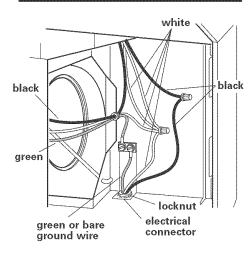
19. Make electrical connections. Install locknut on electrical connector and tighten securely. Connect white to white and black to black wires using twist-on connectors. Connect green or bare ground wire to the green ground screw.
