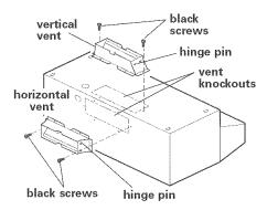
12b. Attach the damper/vent connector to the hood. Use the two black sheet metal screws provided in the parts bag. Note: If wall cap is directly behind vent connector, the dampers in the connector and wall cap MUST NOT interfere with each other. Remove the vent connector damper if they interfere.
