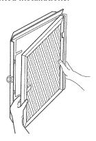
Snap aluminum filter onto front of charcoal filter. Make sure that tab on aluminum filter lines up with finger pull on charcoal filter.
