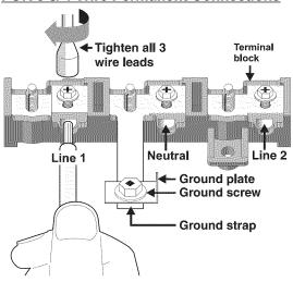
**NOTE:** Non-terminated field wire compression connections must be set at approximately 22in./lbs. Always use 10 ga. wire or larger.
