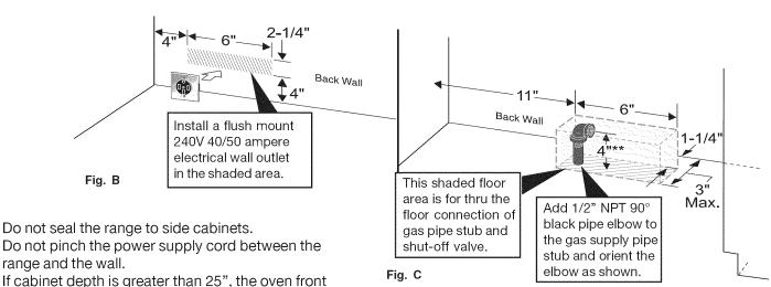
All openings in the wall or floor where the range is to be installed must be sealed.
