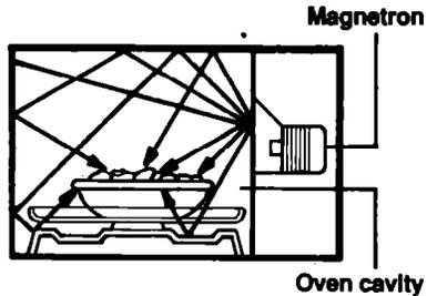
The glass turntable of your microwave oven lets microwaves through. Then they bounce off a metal floor, back through the glass turntable and are absorbed by the food.
