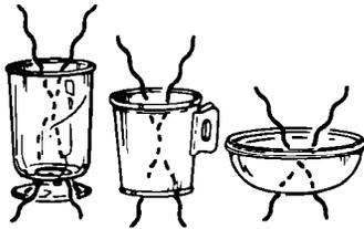
Microwaves pass through glass, paper and most plastics without heating them so food absorbs the energy. Microwaves bounce off metal pans so food does not absorb the energy.
