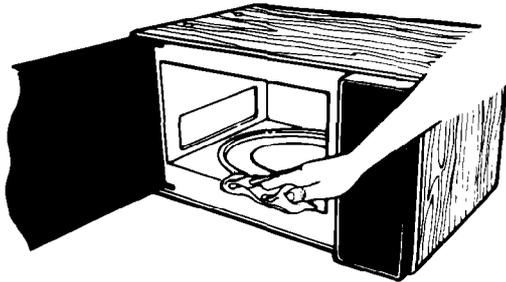
1. Empty the microwave oven and clean inside it with a soft, damp cloth. Check for damage such as misaligned door, damage around the door or dents inside the oven or on the exterior. If there is any damage, please do not operate the unit until it has been checked by an authorized Whirlpool™ service technician and any repairs have been made.
