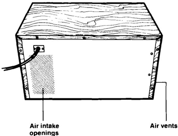
3. **Do not block the rear air intake openings and air vents on side of microwave oven.** Allow a few inches of air circulation on side and back of oven where vents and intake openings are located. Blocking the air intake openings and air vents can cause damage to the oven and poor cooking results. Make sure the microwave oven legs are in place to ensure proper airflow.
