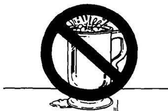
Liquids heated in certain containers (especially cylindrical-shaped containers) may become overheated. The liquid may splash out with a loud noise during or after heating or when adding ingredients (coffee, etc.) resulting in harm to the oven and possible personal injury. For best results stir any liquid several times before heating or reheating.
