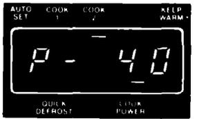
When the Cook 2 cycle ends, "End" will show on the Display and 4 beeps will sound. (You can stop the beeping by opening the door or by touching CANCEL.) "End" will remain on the Display and a reminder tone will sound every 30 seconds (to remind you that food is left in the oven) until the door is opened or CANCEL is touched. The Display will then show the time of day.
