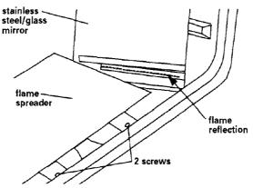
You can check the burner flame by removing the flame spreader or by using a mirror.
