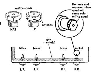
Locate Natural gas orifice spuds in literature package. Remove L.P. gas orifice spuds using a 3/8" combination wrench. Install Natural gas orifice spuds to replace the L.P. gas orifice spuds.
