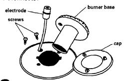
Remove storage drawer and oven racks. Remove burner grates, caps and screws holding burner bases to cooktop. Lift burners off cooktop.
