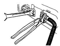
Use 15/16" combination wrench and channel lock pliers to tighten fittings and flexible connector.
