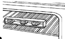
Place rack in oven. Place level on rack, first side to side; then front to back.
