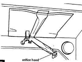
■ Broil burner: Use 1/2" combination wrench to turn the orifice hood down snug onto pin (approximately 2 to 2-1/2 turns). DO NOT OVERTIGHTEN. The burner flame cannot be properly adjusted if this conversion is not made.
