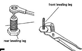
Remove cardboard shipping base from under range. Remove storage drawer. Use a 3/8" drive ratchet to lower rear leveling legs one-half turn. Use channel lock pliers to lower front leveling legs one-half turn.
