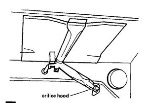
■ Broil burner: Use 1/2" combination wrench to loosen orifice hood away from pin (approximately 2 to 2-1/2 turns). The burner flame cannot be properly adjusted if this conversion is not made.
