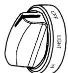
Push in and turn each surface unit control knob to "LIGHT" position. The flame should light within 4 seconds. Turn control knob to "HI" position after burner lights. Do Not leave the knob in the "LIGHT" position after burner lights.
