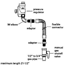
A 1/2" male pipe thread is needed for connection to pressure regulator female pipe threads.
