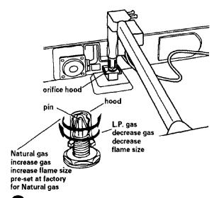
Oven burner: Use 1/2\* combination wrench to loosen the orifice hood away from pin (approximately 2 to 2-1/2 turns). The burner flame cannot be properly adjusted if this conversion is not made.
