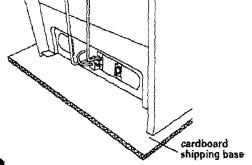
3. Keep cardboard shipping base under range to prevent damage to floor covering.
