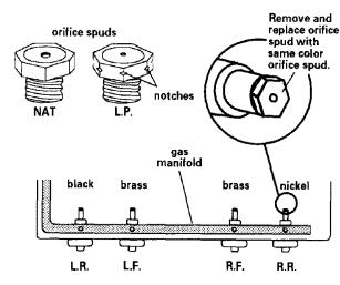
Prop open cooktop maintop. Remove the venturi plates. Locate L.P. gas orifice spuds in a literature package included with the range. Orifice spuds are color coded. Remove one Natural gas orifice spud at a time using a 3/8" combination wrench. Install the same color L.P. gas orifice spud to replace the Natural gas orifice spud.
