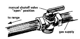
1 1 Check that range regulator shutoff valve is in the "on" position. Open the manual shutoff valve in the gas supply line. Wait a few minutes for gas to move through the gas line.
