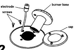
Remove storage drawer and oven racks. Remove burner grates, caps and screws holding burner bases to cooktop.
