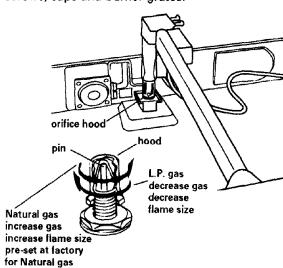
**6** ■ Oven burner: Use 1/2" combination wrench to turn the orifice hood down snug onto pin (approximately 2 to 2-1/2 turns). DO NOT OVERTIGHTEN. The burner flame cannot be properly adjusted if this conversion is not made.
