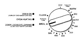
Push in and turn the oven selector control knob to "BROIL." The broil burner should light in 50-60 seconds; this delay is normal. The oven valve requires a certain time before it will open and allow gas to flow.
