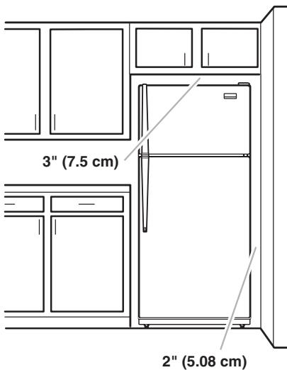
To ensure proper ventilation for your refrigerator, allow for 1/2 in. (1.25 cm) space on each side, 3 in. (7.5 cm) at the top, and 1 in. (2.5 cm) at the back. (At the top, when using half depth cabinet, use top of cabinet height "C" dimension. When using full depth cabinet, use overall "D" dimension.) When installing your refrigerator next to a fixed wall, leave 2 in. (5.08 cm) minimum on hinge side (depending on your model) to allow for the door to swing open.
