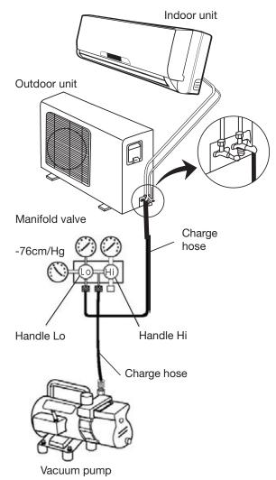
display in the pressure indicator is a little higher than the atmosphere pressure. This procedure verifies if the refrigerant goes through the tubes correctly.
