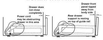
Remove and replace, making sure the power cord is not obstructing the drawer and/or the rail is in the guide.
