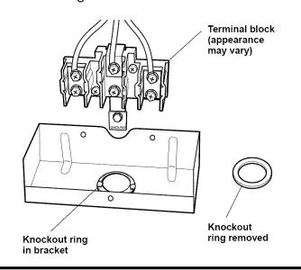
For power cord installations only (see the next step if using conduit), assemble the strain relief in the hole. Insert the power cord through the strain relief and tighten. Allow enough slack to easily attach the cord terminals to the terminal block. If tabs are present at the end of the winged strain relief, they can be removed for better fit.
