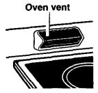
Hot air and moisture escape from the oven through a vent on the lower left side of the backguard. Do not block the vent by using large pans or covers. Poor baking/roasting can result.
