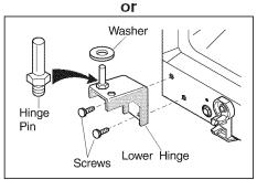
**10.** Turn center hinge upside down and secure to cabinet as shown, using the screws which are in the new holes. Install refrigerator door on lower hinge pin. Align door with edge of cabinet. Hold the door on front of cabinet.
