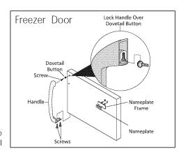
screw and dovetail button, and install on other side, using the same holes as the nameplate. To move nameplate to other side, remove nameplate from its frame, turn frame upside down and install in old handle holes. Insert nameplate into frame. Reverse instructions for reattaching handle. Start with handle offset away from door. Place top of handle over dovetail button, swing handle into an upright position and push upward, locking it into place. Secure bottom of handle with screws.
