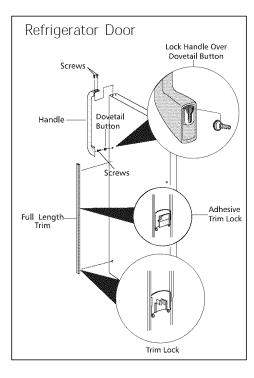
handle offset away from the door. Place bottom of handle over dovetail button, swing handle into an upright position and push downward, locking it into place. Secure top of handle with screws.
