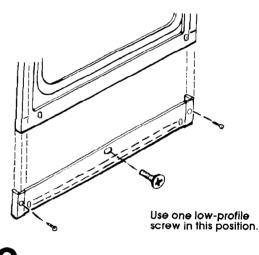
**7** Install the lower vent grille using the three screws provided.
