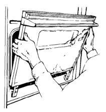
Close lower or single oven door to the broil position. Grasp the sides of the oven door and pull the door up and out of the hinge slots to remove. Set door aside.
