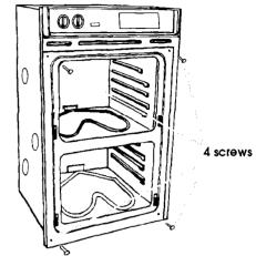
8 Center oven into cabinet cutout. Use two screws (four screws for a double oven) through the mounting holes in the front frame of the oven to secure the oven to the cabinet. Do Not overtighten screws.
