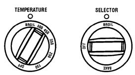
Check the operation of the lower oven broil element. Set the oven selector and oven temperature control knobs to "BROIL." In 1-2 minutes, the upper element should glow red. The lower oven indicator light should be on and the oven should be heating. Turn the oven selector and temperature control knobs to "OFF."
