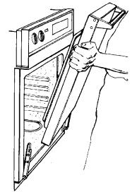
Replace the oven racks. Replace the single oven or upper double oven door by partially fitting the door hinges into the hinge slots. Pull door slightly toward you; then slide door completely in place. Reinstall the two oven-door screws (if required for your oven door). If door does not close, you have not pushed hinges completely into frame. Repeat for lower oven door.
