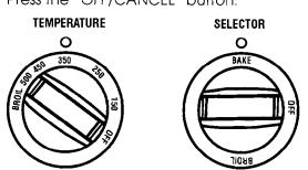
Check the operation of the lower oven. Set the oven selector control knob to \*BAKE." Set the oven temperature control
