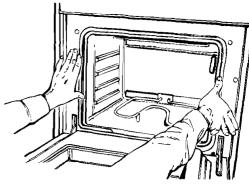
Push against seal area of front frame to push oven into cabinet.
