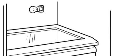
4. Replace the light shield by grasping the top center of the shield and inserting the tabs on one end into the slotted holes in the refrigerator liner. Then, carefully bend the shield at the center to insert the tabs on the other end.
