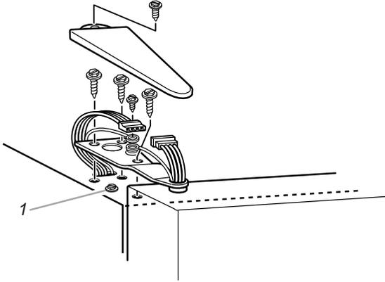
4. Disassemble right top hinge.
