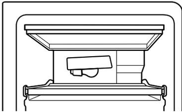
4. Replace the light shield by grasping the top center of the shield and inserting the tabs on one end into the slotted holes in the freezer liner. Then, carefully bend the shield at the center to insert the tabs on the other end.
