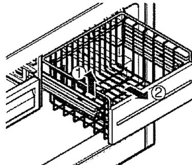
2. To install, pull both rails out to full extension. Hook the basket supports into the rail tabs and push to the back of compartment.
