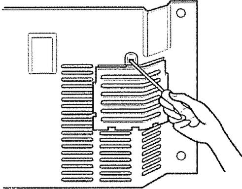
2. Lift off the cover by slightly pushing up
