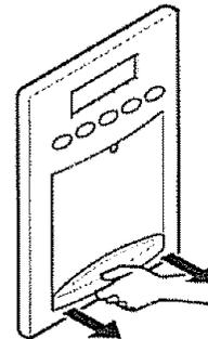
Tilt up the front of tray slightly and snap the ribs into the holes to replace the tray.
