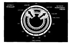
For the first few loads, set the Cycle Control Knob to point to the  $\star$  in either automatic cycle. When the dryer stops, feel the dried items.
