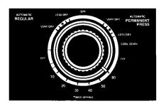
Select a cycle by turning the Cycle Control Knob either way. Stop when the indicator on the knob's outer ring points to the cycle and setting you want. See pages 7-8 for further cycle information.
