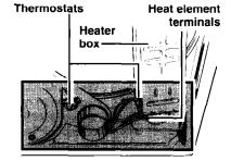
Electric dryer with back panel removed
