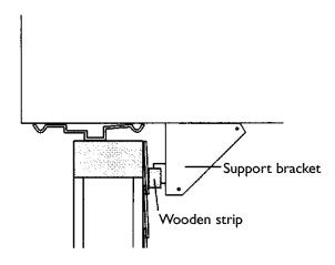
5. Screw or nail cabinet to wooden frame using shims if frame is oversized, to eliminate distortion. Remember to maintain proper slope as described in Step 3.
