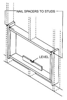
**NOTE:** If wall thickness is 7" (178 mm) or more, add aluminum flashing over bottom of frame opening to assure no water can enter area between inner and outer wall.
