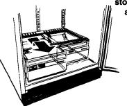
Pull out to the stop, lift the front and pull again.
