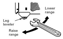
Use an open-end or adjustable wrench to adjust the leveling legs until the range is level.
