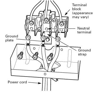
B Re-install the junction block access cover making sure that wires do not become pinched between wire cover and mainback.
