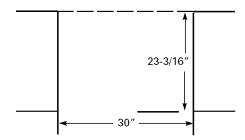
If you have a countertop deeper than 25" and you wish to set the range further back into the counter, the cutout may be cut deeper (up to 24-1/2"), but there must be at least 24-1/2" from the front edge of the countertop and back wall.
