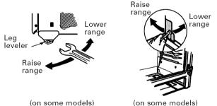
**B** Check for levelness by placing a spirit level or a cup, partially filled with water, on one of the oven shelves. If using a spirit level, take two readings—with the level placed diagonally first in one direction and then the other.
