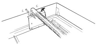
With the oven bottom removed, properly adjusted flames should have approximately 1" blue cones and, if range is supplied with natural gas, should burn with no yellow tipping. (With most LP gas, small yellow tips at the end of outer cones are normal.) Flames should not lift off burner ports. If lifting is observed, gradually reduce air shutter opening until flames are stabilized.
