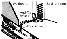
Install the sleeve anchor into the drilled hole and then install the lag bolt through the device. The bolt must be properly tightened as recommended for the hardware.
