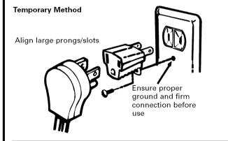
**A** CAUTION: Attaching the adapter ground terminal to the wall receptacle cover screw does not ground the appliance unless the cover screw is metal, and not insulated, and the wall receptacle is grounded through the house wiring. The customer should have the circuit checked by a qualified electrician to make sure the receptacle is properly grounded.
