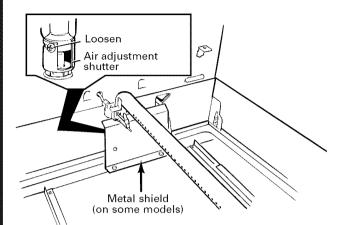
On some models, remove the metal shield at the rear of the cavity. The air adjustment shutter is behind this shield.
