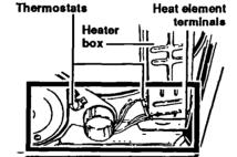
Electric dryer with back panel removed
