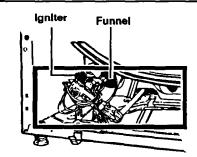
Gas dryer without lower front access panel (full-front panel removed)
