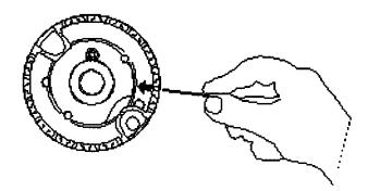
For proper flow of gas and ignition of the burner—DO NOT ALLOW SPILLS, FOOD, CLEANING AGENTS OR ANY OTHER MATERIAL TO ENTER THE GAS OPENING. Gas must flow freely through the small hole in the brass orifice for the burners to light properly. If the gas opening orifice becomes soiled or clogged, use a small-gauge wire or needle to clean. ALWAYS keep the burner cap assembly and ring in place whenever a surface burner is in use.
