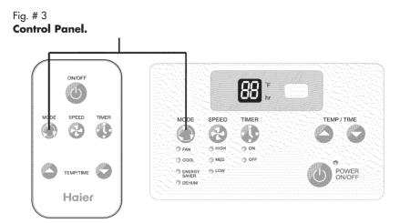
Once the mode function is established, you will have to set the fan speed. (See fig. #4) Every time you press the SPEED button, fan speed will change between LOW, HIGH and MED.
