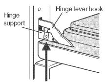
Lock engaged for door removal Figure 1
