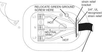
4 #10 AWG MINIMUM COPPER CONDUCTORS OR 120/240V 30A POWER SUPPLY CORD KIT MARKED FOR USE WITH DRYERS & PROVIDED WITH CLOSED LOOP OR SPADE TERMINALS WITH UPTURNED ENDS (NOT SUPPLIED).
