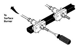
Test to verify if "LOW" setting should be adjusted
