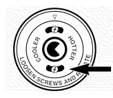
Back of the OVEN TEMP knob. Lower screw moves toward hotter or cooler.
