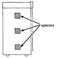
Attach three spacers from the miscellaneous parts bag to the top, middle and bottom of each side of the refrigerator. Spacers are required for ventilation.
