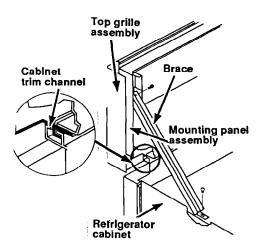
Attach the brace to the top right front corner of the refrigerator cabinet with one screw. Insert top grille flange into cabinet trim channel and align grille with top and side trim. Attach top grille mounting panel assembly to brace with one screw. Fasten grille in place with six screws.
