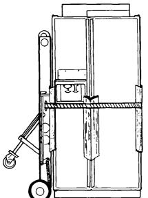
Place appliance dolly under the side of the refrigerator. Wrap strap from truck
