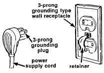
Move refrigerator close to final position. Remove cardboard or plywood from under refrigerator. Plug electrical cord into the grounded outlet. Use the screw from the parts package to install the plug retainer. Move the refrigerator evenly and straight into the opening. Check that the water line will not be kinked. Check that slack in the electrical cord hangs freely behind refrigerator or is placed on top of refrigerator next to cover.
