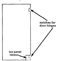
4. Height of side panels depends on your installation site. Side panels may need to be notched to clear door hinges. Side panels may be cut to match toe panel recess if desired.
