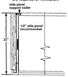
A side panel support nailer should be attached to the rear wall on each side of refrigerator
