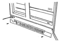
15. Open both doors. Use two screws to attach bottom grille to cabinet.
