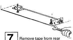
Remove tape from rear leveling rods. Turn the two leveling rods clockwise using a 5/16" socket and ratchet until the cabinet weight is supported by the rear legs. Use 1-3/8" open end wrench to lower the front leveling legs until the weight of the cabinet is supported by legs.
