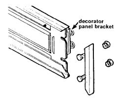
Remove two nuts from one end of the top panel frame. Remove end piece. Slide decorative panel into panel frame. Replace end piece using nuts.
