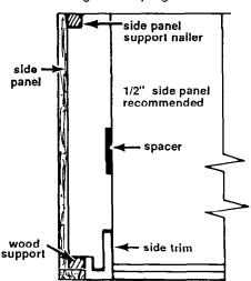
If less than 25" depth is available, side panel installation will need to be completed according to each site's restrictions. One method is to attach side panel to outside of side trim. However, this will increase width required. Drill holes into side trim. Attach a wood support to side trim. Attach side panel to panel support nailer and wood support. Cover wood support with a panel piece to match side panel.
