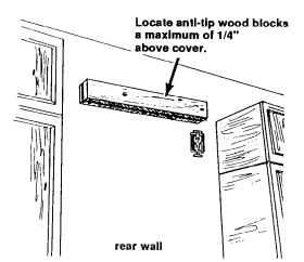
When a soffit is not available, locate wall studs in the refrigerator opening. Center one wood block and use wood screws to attach the wood block to the wall studs. Make sure screws engage wall studs a minimum of 1-1/2". Screw the second wood block to the front of the first block. The wood blocks must extend 2 inches beyond the ends of the cover.
