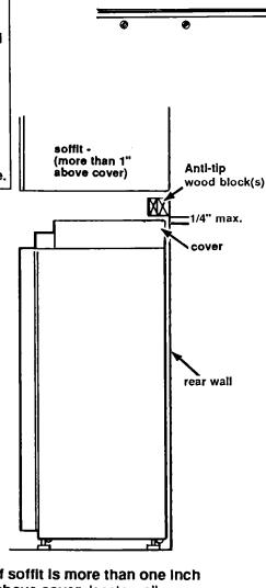
If soffit is more than one Inch above cover, locate wall studs in the refrigerator opening. Center one wood block and use wood screws to attach the wood block to the wall studs. Make sure screws engage wall studs a minimum of 1-1/2". Screw the second wood block to the front of the first block. The wood block(s) must extend 2 inches beyond the ends of the cover.
