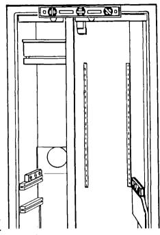
Refrigerator must be level for proper operation. Important:
