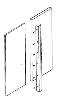
Remove all tape and door bracing from refrigerator door. Remove the six screws that attach the handle to the door frame. Slide the refrigerator door panel into door frame. If the panel is less than 1/4" thick, a filler panel will need to be installed between the door and decorative panel. If the decorative panel is more than 1/4" thick, it will have to be routed to have a 1/4" edge on all sides. See Custom panel and insert dimensions for exact sizes to cut custom panels.
