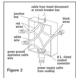
If local codes PERMIT connecting cooktop-ground conductor to neutral junction box wire: (three-wire system)
