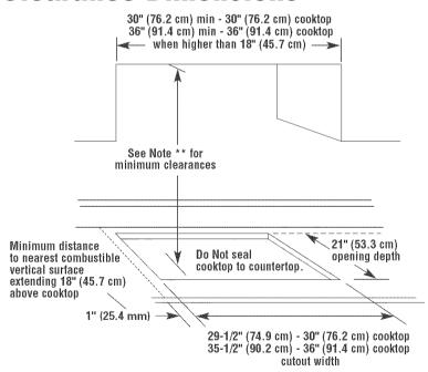
**Side clearance** — 6" (15.2 cm) minimum clearance between side of cooktop and side wall is recommended for maximum ventilation performance.
