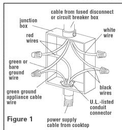
If local codes DO NOT PERMIT connecting cooktop-ground conductor to neutral white wire in junction box: (four-wire system)
