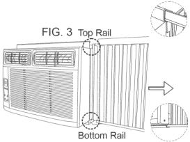
Your air conditioner is designed to install in standard double hung windows with opening widths of 23 to 36 inches (584 mm to 914 mm) (FIG. 4A , FIG. 4B).
