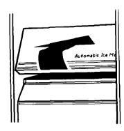
Lift the signal arm so it clicks into the OFF (up) position. Ice can still be dispensed, but no more can be made.
