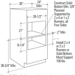
Note: Additional clearance between the cutouts may be required. Check to be sure the oven supports above the Warming Drawer location does not obstruct the required interior 23-1/2" depth and 9-1/4" height. See installation instructions for details.
