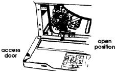
The dryer shutoff valve is located behind the lower front access panel. The wiring diagram is located inside the console. If necessary for service, open the access panel by pushing down on the locking clips with a small, flat-blade screwdriver, and pulling panel forward. The clips are located on top of the panel 3 inches (7.6 cm) in from each side. The panel is hinged at the bottom. Close the access panel after servicing. Do Not operate the dryer with the access panel open.
