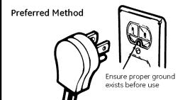
The power cord of this appliance is equipped with a 3-prong (grounding) plug which mates with a standard 3-prong grounding wall receptacle to minimize the possibility of electric shock hazard from this appliance.
