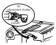
The air adjustment shutter for the top (broil) burner is in the center of the rear wall of the oven.
